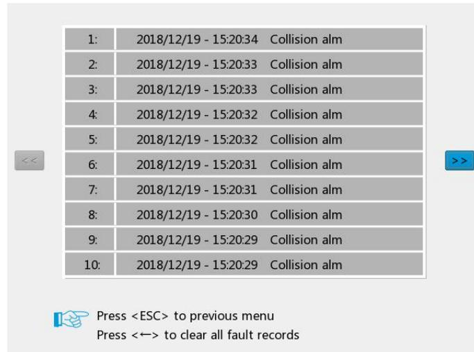
The interface can record the alarm information generated during the movement, so that the user can troubleshoot the fault and save up 20 alarm information. Press the [←] button on the panel to clear all alarm records.
