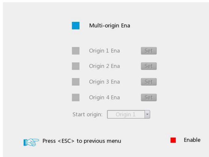
At this time, the blue cursor defaults to the [Multiple Position Enable] option. Press [enter] to select or cancel the entry. When multiple anchor points are enabled, first move the blue cursor to [Origin 1 Enable] .Press the [enter] key to enable the option, then press the [Right] key to select the [Set] option and press the [Enter] . The interface as following interface:
