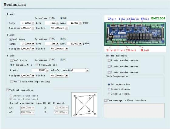
Select drive mode for Y axis (single drive or double drive), based on mechanical structure, and then configure information of rotation axis.
