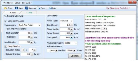
When inertia ratio is less than 200 percent, the device is light loaded, and enables high-speed cutting.
