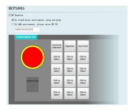
BCP5045 numerical control panel can be activated in numerical control panel interface. When used in a stand-alone environment, CypCut software will adaptively match the Mac address of BCP5045 numerical control panel, and automatically connect the control. When BCP5045 is used in LAN environment, please enter BCP5045 device ID number. BCP5045 is in total of 12 custom keys, which can be configured as a control button of double exchange workbench or other custom PLC.
