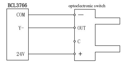
Typical connection of contact switch is shown as below: o
