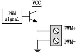
We strongly recommend that users install PWM+/- signal to a relay output port in series (Set it to PWM+/- enable signal.), then access to the laser, which can avoid laser light leakage in modulation mode. Please refer to "2.5 Laser Connection" for more details. Furthermore, please adjust PWM signal level. 24 V or 5 V level can be selected through dip switch.
