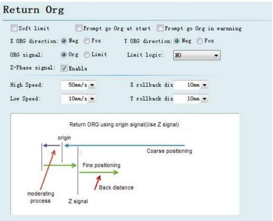
As long as conditions allow, be sure to select "Use Z signal", which will greatly enhance the accuracy of homing origin. BMC1604V2 motion control card matched with CypCut provides encoder input to each axis, to extremely ensure accuracy.
