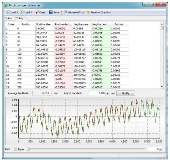
Click "Import X", which can import X-axis error data, and click "Import Y" which can import Y axis error data. The imported results will be displayed in lists and graphics after data completion.
