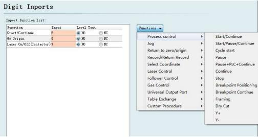
Click on the "Function Select" button, users can select the function name of the input port in the drop-down list, and then configure the corresponding input port and level detection.
