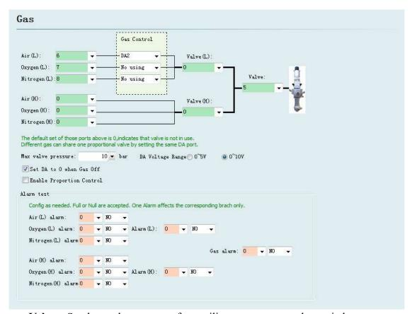
**Valve:** Set the total output port for auxiliary gas correspond to switch.
