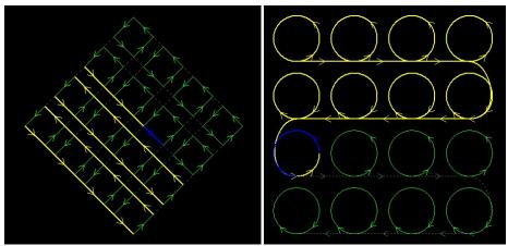
2. Naturally successive cutting of arc: After the circle array is selected, set as naturally successive cutting of arc. Actual cutting is the same as connecting all circle or arc with a straight line. There's no acceleration and deceleration during processing, with just opening and closing the light.
