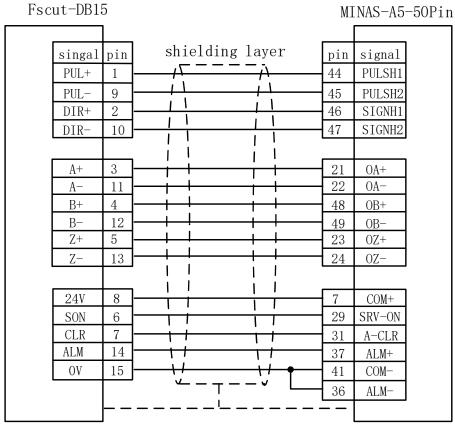
The wiring diagram of Panasonic A5 low-speed pulse
