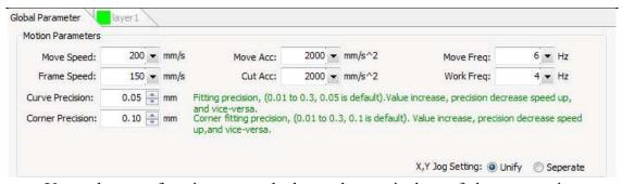
Use pulse test function, test whether pulse equivalent of the system is set correctly or not, click to test whether the direction and motion of each axis is normal or not.
