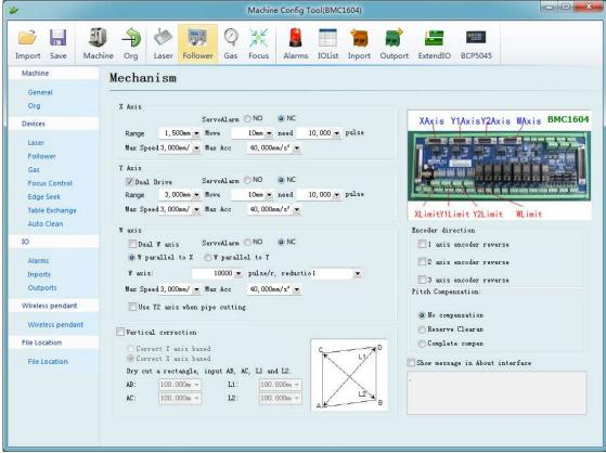
Main interface of platform configuration tool is information overview; The left and the upper convenient buttons are for entering various parameters setting page; green selected box as shown in the figure above is convenient button for controlling laser, height controller and adjusting auxiliary gas. Click left "config file" button to locate Data file.
