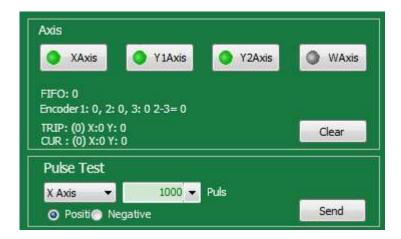
3. If the pulse feedback transmitted forward is negative, enter "the platform configuration tool - Machine page" to reverse the encoder corresponding to the number of axis. (Note: Have to set synchronously the encoder feedback of the second shaft and the third shaft in case of double-drive machine).
