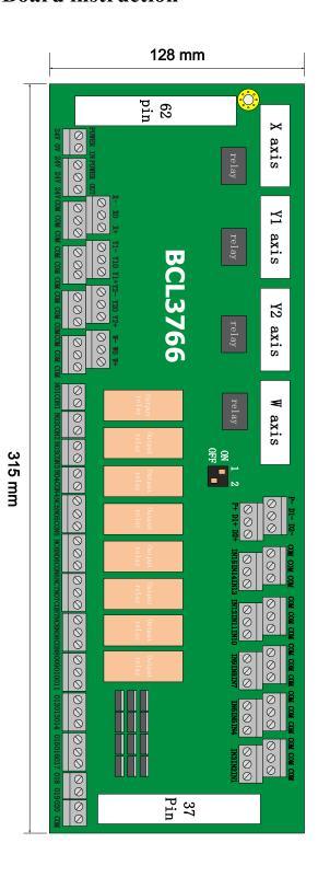
The External IO Board of BCL3766 is installed by rail and also can be installed permanently. Its external size is 315mm\*128mm with DM62M and DB37M interface in two sides, corresponding to JP1 and JP2 of BMC1604V2. C62-2 cable is used to connect External IO Board DB62 interface with JP1 port on the back of control card JP2 interface is linked by C37-40 baffle wire and then is fixed on erection fixture of computer with bolts. And C37-2 cable is used to connect DB37 socket on External IO Board.
