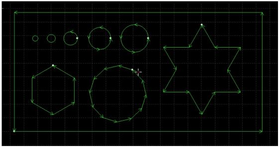
Adjust the FIR frequency as high as possible in the case of no affecting the accuracy. It is required the corner does not generate waves when cutting a rectangle, polygon and star. It can be set according to experienced value of the following table, Or debug the FIR frequency within the upper and lower two ranges after determining a processing acceleration. These two parameters, processing acceleration and FIR
